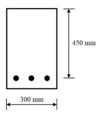
As per Limit State Design of IS 456:2000, the design moment capacity (in kN.m, round off to two decimal places) of the beam section, is \_\_\_\_\_\_.
