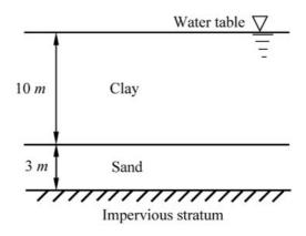
The settlement (in mm, *round off to two decimal places*) of the clay layer, 10 years after the construction of the fill, is
