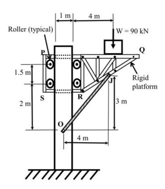
The magnitude of horizontal component of the reaction (in kN) at pin O, is
