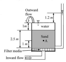
The effective stress (in kPa, round off to two decimal places) at point A, located 1 m above the base of tank, is \_\_\_\_\_\_.
