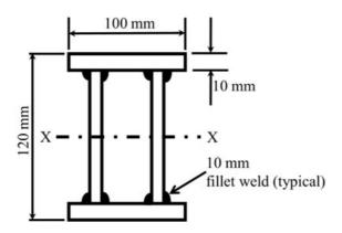
The maximum shear force (in kN, round off to one decimal place) that can be carried by the section, is
