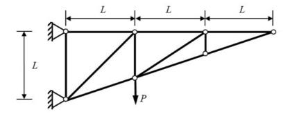
Neglecting self-weight of the members, the number of zero-force members in the truss under the action of the load P, is
